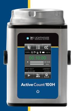
ctiveCount100H is a high performance portable active air sampler suitable for use in cleanrooms and aseptic environments. The ActiveCount100H is truly ISO 14698 compliant with a d50 collection efficiency of 1 micron and HEPA filtered exhaust ports designed to avoid re-aspiration of sampled air.
